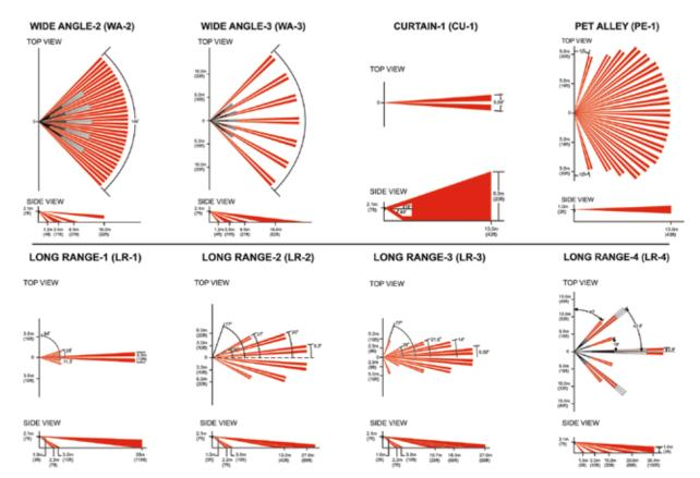
The beam patterns represent the optional lenses that are available for the 476+, DG55, DG65 and 525D motion detectors. Distances shown may vary according to the selected motion detector.
